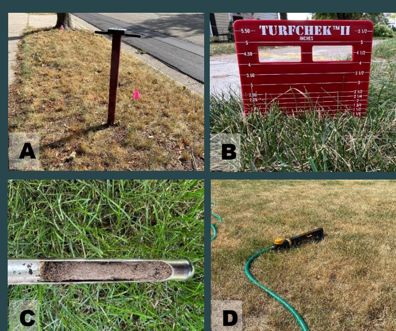
Figure 3. (A) A portable soil moisture sensor in a boulevard sampling location. (B) A turfgrass height of cut gauge. (C) A soil sample pulled from a lawn. (D) A portable sprinkler on a lawn.
