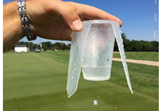
MEASURE THE DEPTH OF WATER (inches) IN EACH CAN
